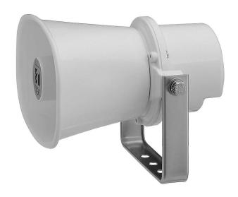
The SC-610M is a compact, highly intelligible speaker suited to public address announcement applications. Its external speaker component finished with powder coating, and stainless steel bracket and screws ensure the unit's weatherproof capability.
