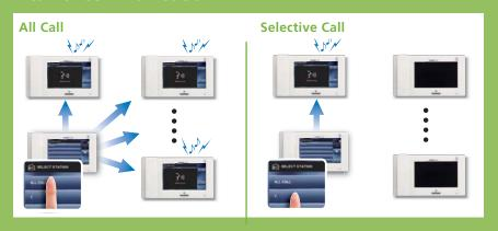
Easily communicate between stations. Simultaneously make an announcement to all inside stations or select a single station to call.
