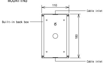
Built-in back box dimensions; 180H x 110W x 45D. Secure opening with a space of 2mm between each side of box and wall.
