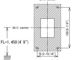
\* Opening cut out for single-gang wall mounting : H70(2-3/4") x W50(1-15/16")
