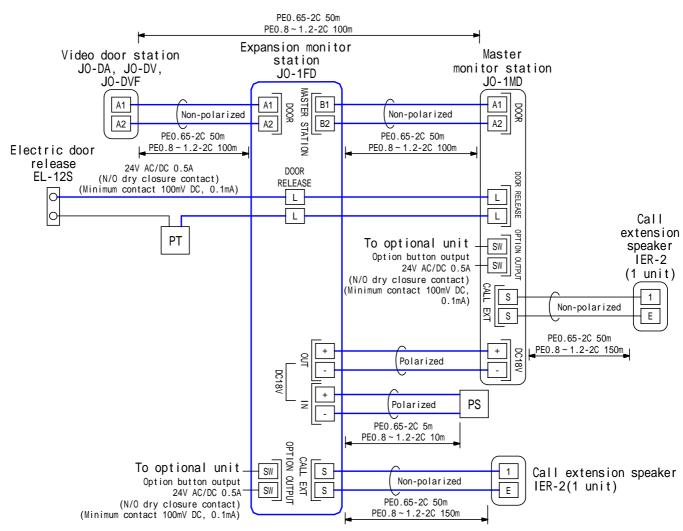
PS : 18V DC, PS-1820UL, PS-1820D, PS-1820 or PS-1820S power supply
