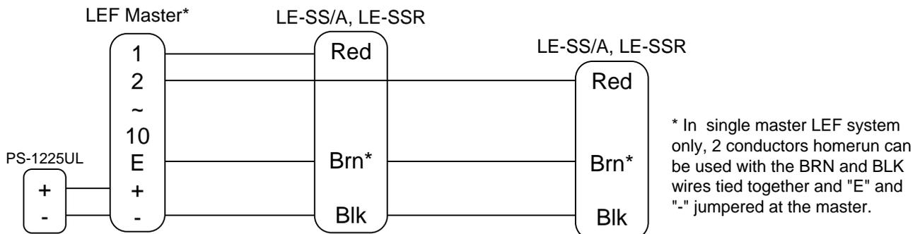
Ensure correct polarity is observed when wiring the sub station. If Brown and Black wire connections are reversed (Black wired to E and Brown wired to negative), the master station will not ring when the call button is pushed but communication will still work normally.
