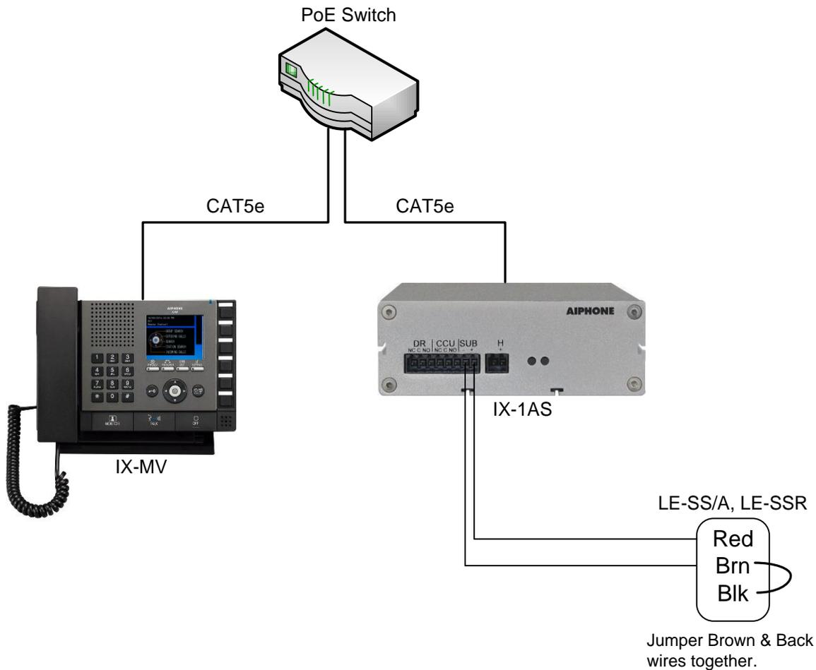
Intercom wiring must be run at least 20" away from any AC wiring, fluorescent lighting, dimmer switches, or any other electronic device that may cause interference.
