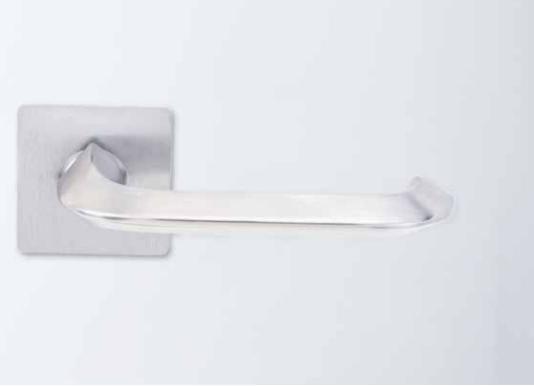
The 260SQ Series door furniture has a 55mm x 2mm square rose. Concealed fixed plates have studs with internal threads located on the rose, visible roses have corresponding countersunk holes and are fixed back to back through the door.
