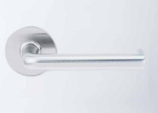
The 260 Series door furniture has a 55mm round rose. Concealed fixed plates have studs with internal threads located on the rose, visible roses have corresponding countersunk holes and are fixed back to back through the door.
