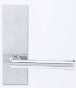
The 224 Series Door Furniture is 162mm long x 50mm wide with square ends. Concealed fixed plates have studs with internal threads located top and bottom, visible fixed plates have corresponding countersunk holes and are fixed back to back through the door.
