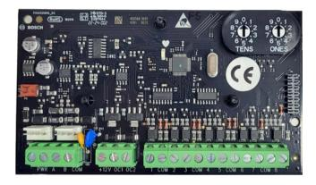
The B228 8-Input, 2-Output Expansion Module is an 8 points/zones supervised expansion device with 2 additional switched outputs that connects to control
