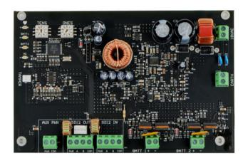
The B520 Auxiliary Power Supply Module is a fully supervised, addressable SDI2 bus device that provides an integrated auxiliary power supply solution for Bosch control panels.
