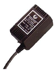
Includes built-in thermal fuses that will blow during overload or fault conditions, eliminating possible fire threat from excessive heat building up inside the casing. The TF008 incorporates a three-wire flying lead that enables a mains earth connection to be made between the equipment and the transformer. This connection might be required for lightning protection on equipment connected to telephone lines or for safety reasons such as earthing of metal enclosures.
