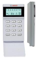
The ICP-CP500ALW is an eight-zone LCD codepad that is compatible with certain Solution Series control panels. Easy to recognize icons display system conditions in a simple to view format. Zone status is indicated numerically across the top of the screen. The codepad notifies you when a zone is unsealed, when there has been an alarm, and in which zone the alarm has occurred.
