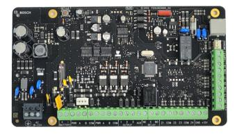
ICP-SOL4-P control panel with door control is for small to medium residential and commercial applications.
