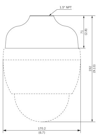
Fig. 3: NDA-4020-PIP Pendant interface plate
