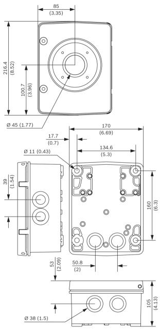
*Fig. 2:* NDA-U-PA0 Surveillance cabinet 24VAC NDA-U-PA1 Surveillance cabinet 120VAC NDA-U-PA2 Surveillance cabinet 230VAC
