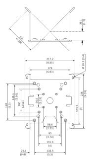
Fig. 5: NDA-U-CMT Corner mount adapter
