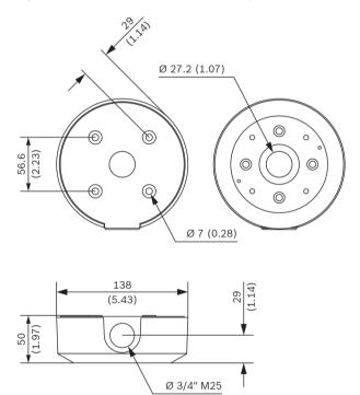
Fig. 6: NDA-U-PSMB Pendant wall/ceiling mount SMB
