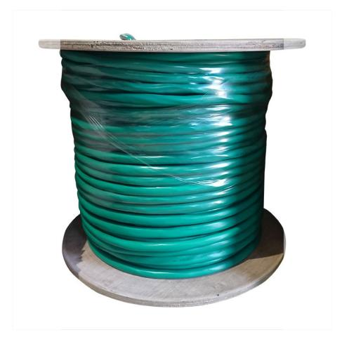
The APAC200G is an all-in-one composite cable, specifically designed for access control systems. The cable consists of 1 x 6-Core access control cable, 1 x 4-Core & 6-Core alarm cables, and 1 x Figure 8 power cable, all encased in a thick green outer sheath.
