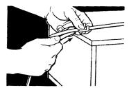
Thread the strap through the seal the second time, completing the loop. About a four-inch length of strap should protrude through the seal.
