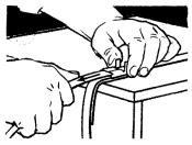
Pull strap tightly around box and through seal. Note 1-inch distance between seal and box edge, also correct position of underflap.
