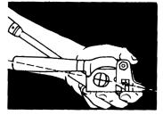
6. Hold tool in left hand as shown. Line up slots in the nose and ratchet so they are on a straight line, as indicated by the dashed line.
