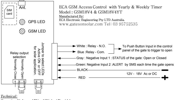
Operating Voltage: 12V – 18V Ac / Dc. / 1Amp Size: 70W x 105L x 25D mm GAM 3G 4G Mini SIM card.
