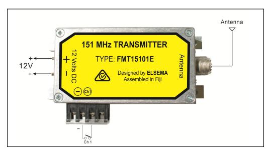
Inputs of the transmitter should be voltage free contact closure only.
