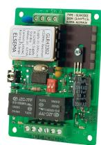
When programming is completed and the GIGALINK cable is removed from the multi channel receiver-coding socket, the 2-way dip switch is used to select different output modes. This is described below.
