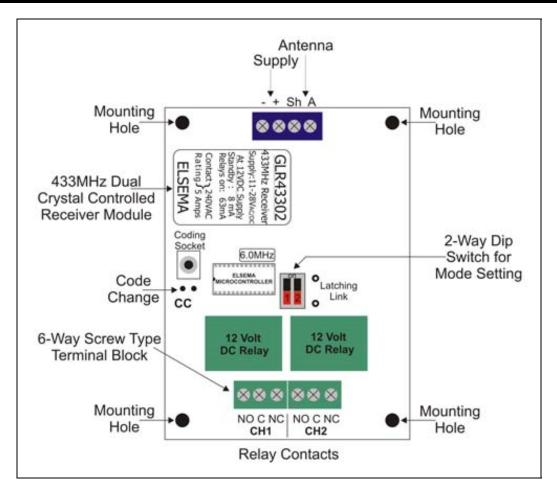
Sh terminal is used for antennas with coaxial cable. The shield (braid) on the coaxial cable should be connected to the Sh terminal while the core of the coaxial cable is connected to the A terminal.
