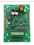
MCR91503R 3-Channel 915MHz Receiver with **Relay** Output
