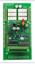
MCR91512SS 12-Channel 915MHz Receiver with **Open Collector** Output
