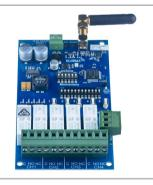
PCR43305R 5-Channel Receiver with Relay Outputs
