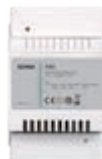
6582 Additional supply unit for LED and cameras, 10,5 Vdc, 13,5 Vdc and 18 Vdc, 230 V~ 50/60 Hz 35 VA 6582/240 As above, 240 V~
