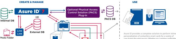
personalization of contactless smart cards for a variety of uses during the print process. Whether you combine cardholder data from various sources using the Live Link real-time data exchange for cashless vending applications, or registering the card information into a physical access control solution so that it can be used for door access, Asure ID has you covered.
