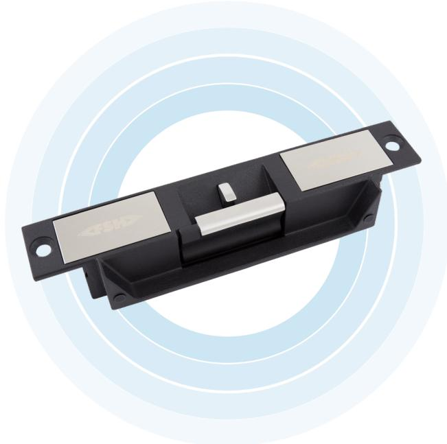
The patented FES20 Series high security electric strikes are manufactured from stainless steel, accept voltages from 11 to 30VDC and have a simple and unique Power To Lock (PTL) / Power To Open (PTO) field interchangeable mechanism, with no loose screws or pins.
