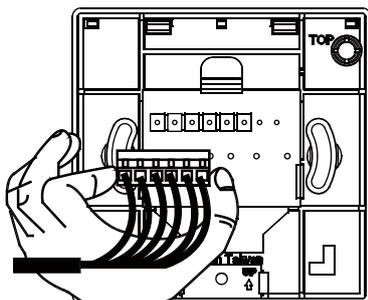
The CP-33 series with Detachable Terminal Blocks is designed with convenient terminal block concept for easy and quick installation. Simply wire the terminal connector and plug it in the back of the CP-33 product. No re-termination is required.
