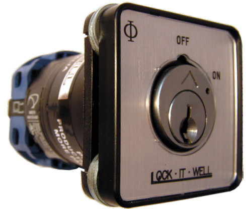
The Example shown is for a R-Series Lockwood 6-pin inline, Panel mount, with key removal in 2 positions at 240V at 20 amp switch.
