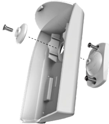
FIG 2. Installation of the Standard Swivel Bracket.
