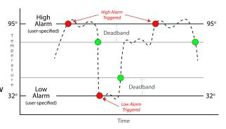
Deadband ensures that once the high alarm is triggered, it won't trigger again until the temperature first drops below 94 degrees (95 - 1).
