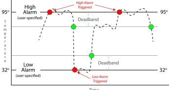
trigger again until the temperature first drops below 94 degrees (95 - 1).
