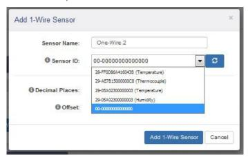
Enter a descriptive name for the sensor in the *Sensor Name* box such as "Outdoor Temperature". The text in this field appears to the left of the corresponding temperature/humidity reading on the Control Page. This text also appears in the email status message when email notifications are enabled. When later defining the control logic, logging and other settings, this label appears in the pull-down lists of sensor resources. This field can be up to 27 characters in length.
