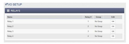
Click the respective *Edit* button to configure each relay. Local relays have some settings that remote relays don't have and vice versa.
