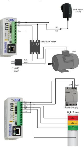
When mechanical relays switch inductive loads such as motors, transformers, relays, etc., the current will arc across the internal relay contacts each time the contacts open. Over time, this causes wear on the relay contacts which can shorten their life span. When switching an inductive load, it is recommended that relay contact protection devices are used.
