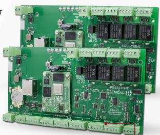
195mm x 107mm x 31mm 11.5 - 14.5V D.C. @ 1A On-board CM4 computer Industry standard connectors NIDAC peripheral bus No jumpers to configure reader devices (Rev. 3 hardware shown)
