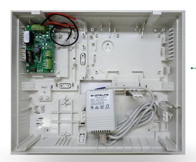
Enclosure 13.8VDC 1.5A battery back up 16VDC Plug pack
