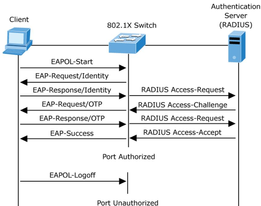
Figure 4-5-2-2: EAP Message Exchange
