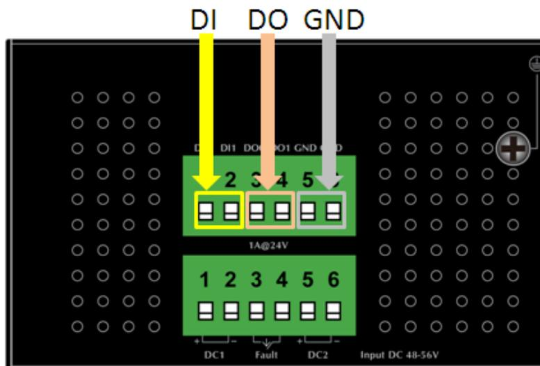
Figure 2-15 Wiring the Redundant Power Inputs
