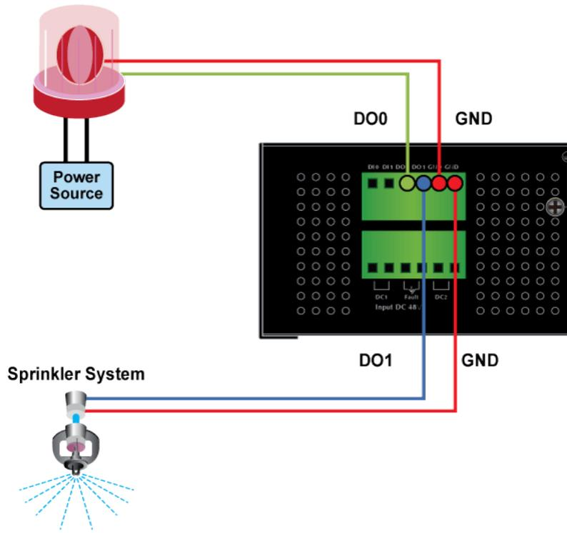
**Figure 2-18** Wiring DO0 and DO1 to Open Detector
