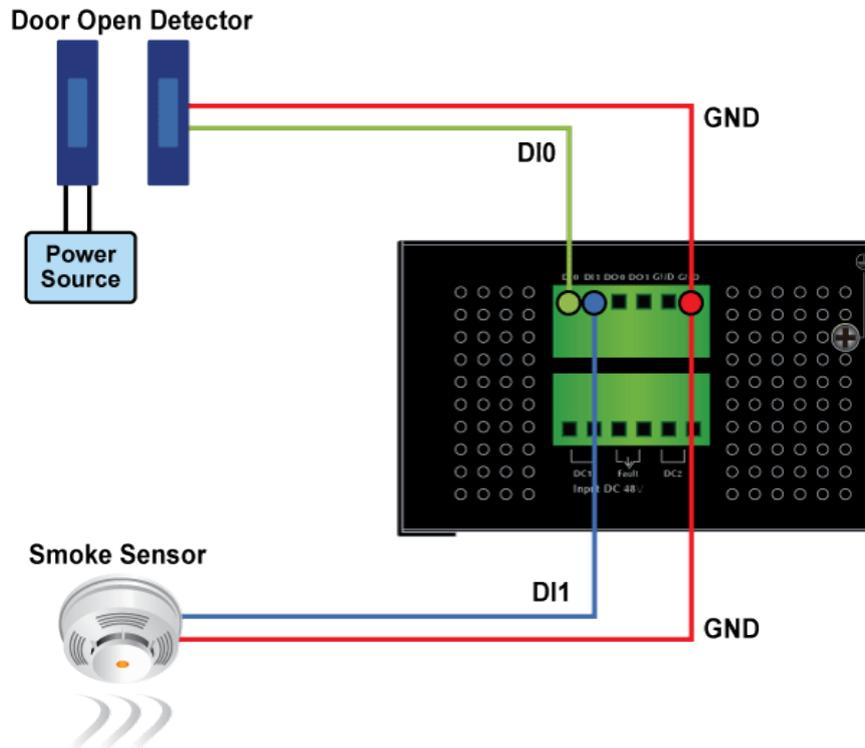
**Figure 2-17** Wiring DI0 and DI1 to Open Detector
