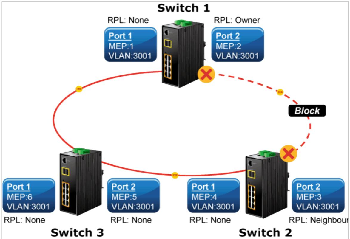
Figure 4-7-1-6: Ring Example Diagram
