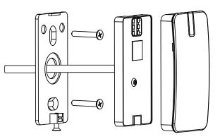
0. Make small recess or hole (diameter is 14 mm) to connect cable under the reader's case.
