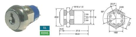
Panel hole 19mm. 33.6mm overall depth. 61mm depth with key inserted, including terminals. Two keys supplied. Rated 2A @ 250V ac, 4A @ 125V ac, 4A @ 28V dc.
