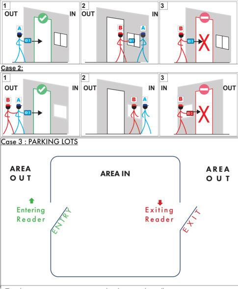
This drawing represent an antipassback secured installation:
