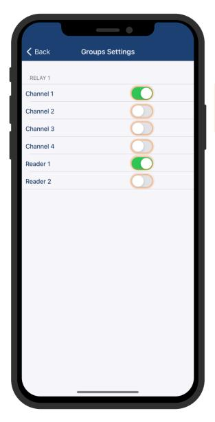
Define the association of each radio channel and/or readers with the selected relay (here RELAY 1)
