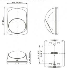
The passive infrared sensor is designed to detect infrared energy variations caused by the presence of a human body. Therefore, note that similar variations in conditions in protected area, due to other reasons, may cause the sensor to create an alarm as it is unable to distinguish between sources
