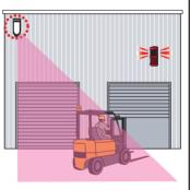
Installing the sensor in a high position will not obstruct the path of vehicles for traffic reminder systems.
