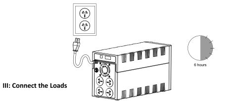
Plug in the loads to output receptacles on the rear panel of the UPS. Turn the power switch of UPS on, then turn connected devices on All units connected to the UPS will be protected by the UPS.
